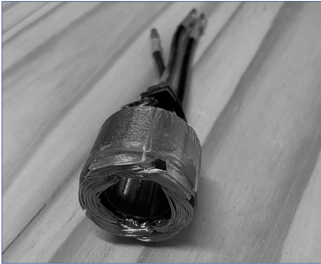
Figure 8. The induction stator coil of a brushless motor driven by three-phase power with the cylindrical rotor removed, that normally rotates outside of the coil.
